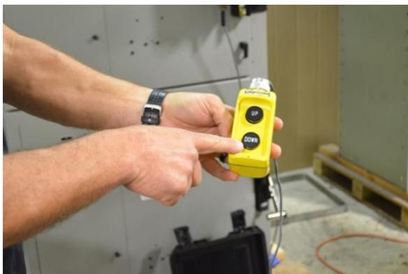
UP button will move the operator arm in an Upward direction towards the "ON" position.
