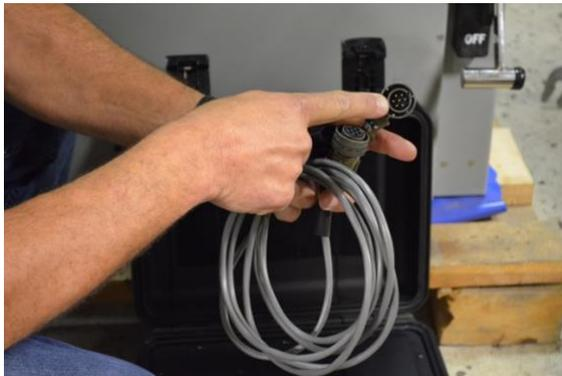
**Place the isoRAC® Control Box on the floor or work table near the unit being racked. Locate the 7 pin interconnect cable, and attach the 90 degree Male connector to the corresponding female connector on the Control Box. Twist the collar ¼ of a turn to ensure positive connection.**
