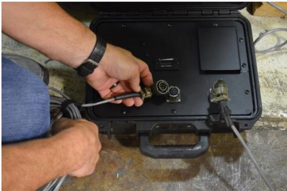
**Insert the 5 pin – 90 degree male end into the corresponding female connector on the Control Box.**
