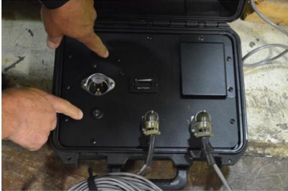
Once all connections are made turn the Power Switch to the "ON" position.
