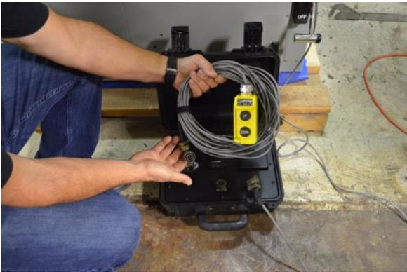
**Locate the Operator Pendant Station with the 5 pin -90 degree plug.**
